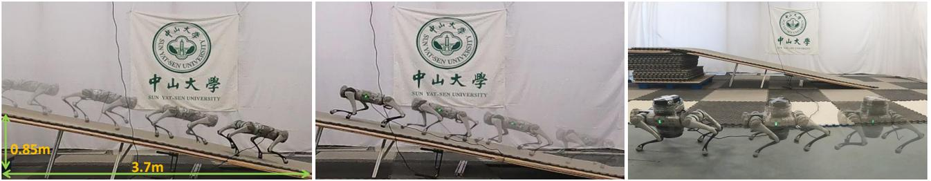
Fig. 7: Experiments. Left: Downhill trotting. Middle: Uphill trotting. Right: Trotting with an 11 kg payload at 0.8 m/s.
